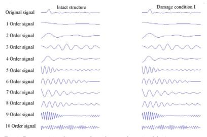
Fig. 2. Decomposition diagrams of wavelet transform signal for intact structure and damage condition I
